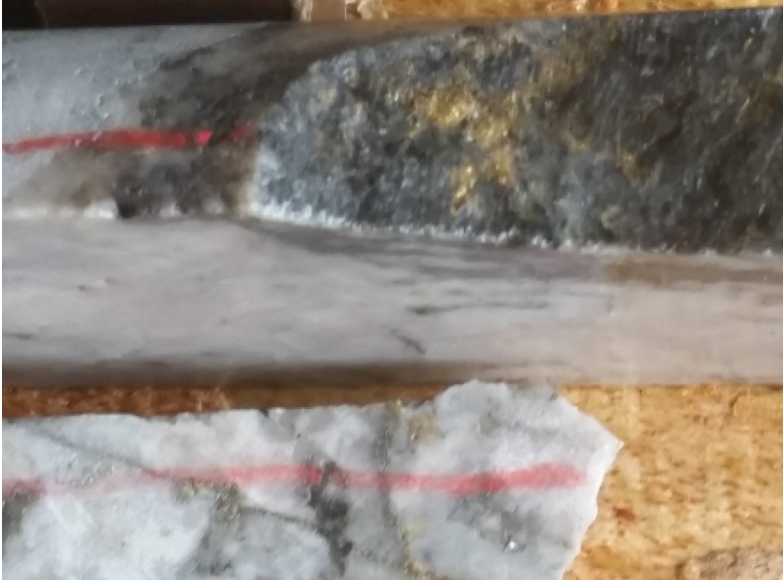
Figure 4:: Visible Gold in Drill Core; sulfides above and quartz below
