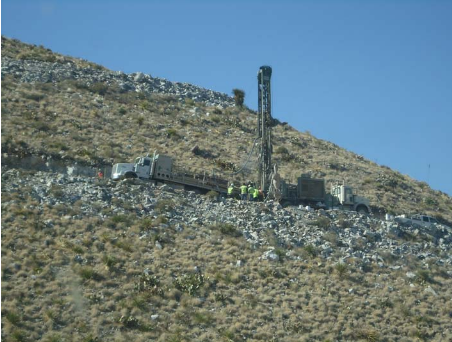
Figure 1: Reverse Circulation Rotary Rig Working on Round Top November 3, 2011
