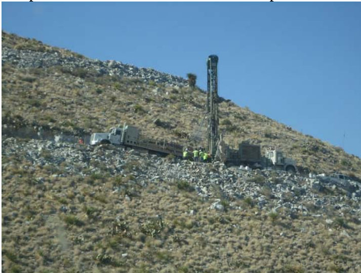
Figure 2: Reverse Circulation Rotary Rig Working on Round Top November 3, 2011; (Because rock so fractured, TRER uses rotary rig as it does not expect competent diamond core recoveries if it spent extra dollars on diamond drill holes).
